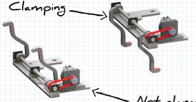
This is the most common pallet hook version. It operates with a rotating cylinder that via a belt rotate the pallet hooks normally 180 degrees. This makes the footprint no larger than the tool and is also possible to use on UniGripper LayerGrippers that are of full pallet size.
